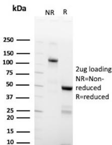
SDS-PAGE Analysis of Purified Myc proto-oncogene protein Recombinant Rabbit Monoclonal Antibody (MYC/7683R). Confirmation of Purity and Integrity of Antibody.
