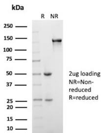
SDS-PAGE Analysis of Purified PSA Mouse Monoclonal Antibody (SPM352). Confirmation of Purity and Integrity of Antibody.
